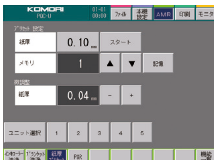
Sheet thickness preset on touch-panel operation screen
